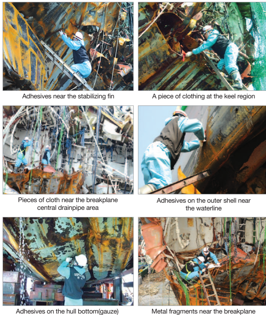
〈Figure III-2-4〉 Evidence collection at the bow
