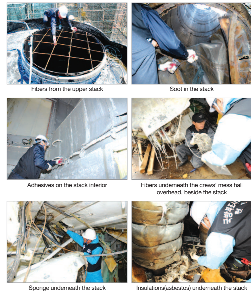
〈Figure III-2-5〉 Evidence collection at the stack
