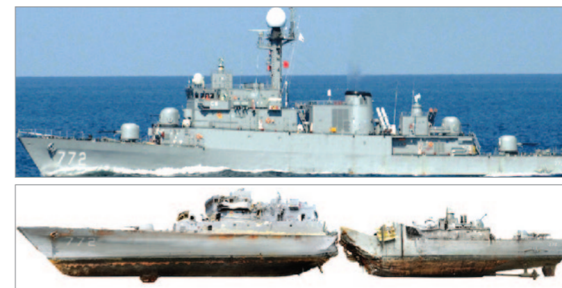
<Figure II-2-1> Shape of damage on ROKS Cheonan
