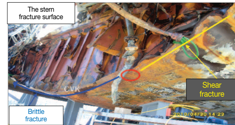
<Figure Appendix III-2-2> The pattern of fracture on the stern
