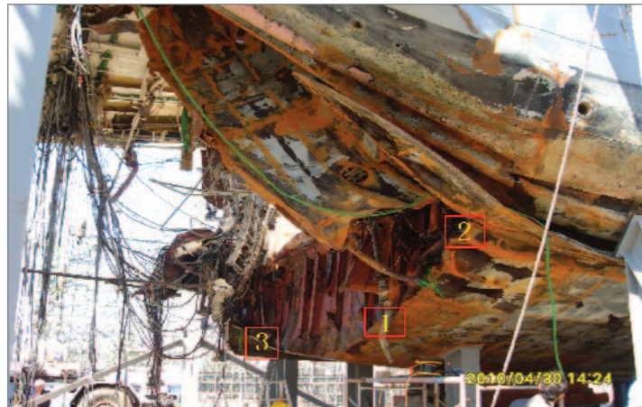
<Figure Appendix III-1-1> Sample collection locations at breakplane
