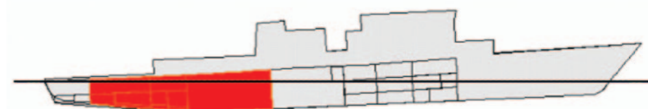
〈Figure Appendix VI-4-4〉 Buoyancy level with three compartments flooded(Case 3)
