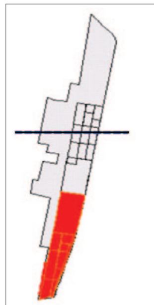
〈Figure Appendix VI-4-7〉 Buoyancy level with four compartments flooded(Case 6)
