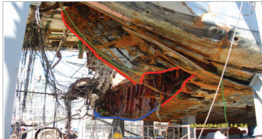
<Figure Appendix III-2-3> Overall fracture pattern of the stern part
