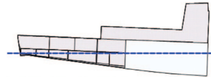
<Figure Appendix VI-5-2> Estimation of the stern buoyancy level immediately after the separation
